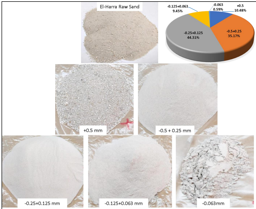
Fig. 6. Photographs show different fractions of dry sieving analyses and their corresponding mass percent of the El-Harra raw sand
